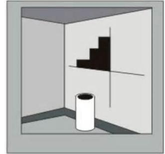
For diagonal installations, it is recommended to follow a similar method as above (by finding the center point of the wall), but instead of relying on horizontal and vertical lines, you will draw diagonal lines at 90 degrees to one another. Once these diagonal chalk lines are drawn, you then need to determine in which direction you want the Stick Bricks to be oriented (either along the left line, or the right line).
